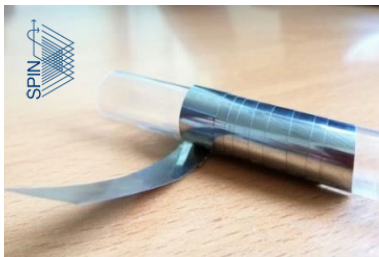
A metallic biaxially textured substrate developed at CNR-SPIN for the deposition of IBS coated conductors
